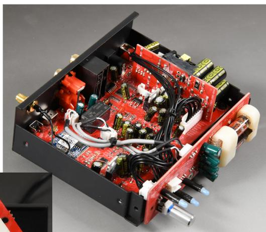
Raytheon 5703 subminiature tubes are mounted on a fixed insulating support.
